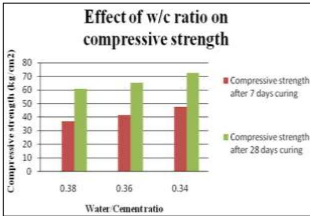
Figure.1. Compressive strength v/s water cement ratio at A/C = 5
