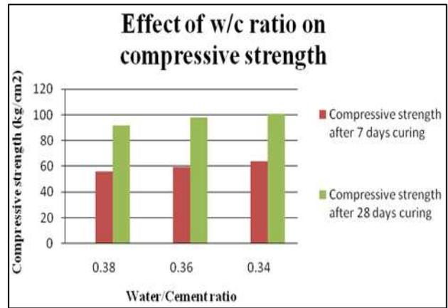
Fig. 3: Compressive Strength v/s Water Cement Ratio at A/C = 4
