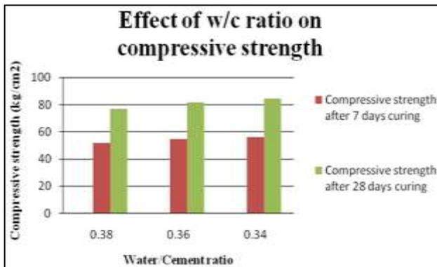
Fig. 2: Compressive Strength v/s Water Cement Ratio at A/C = 4.5
