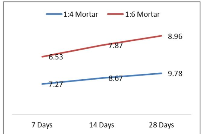
Fig. 7: Comparison of compressive strength of 1:4 and 1:6 cubes with bottles arranged Perpendicular to the direction of load application
