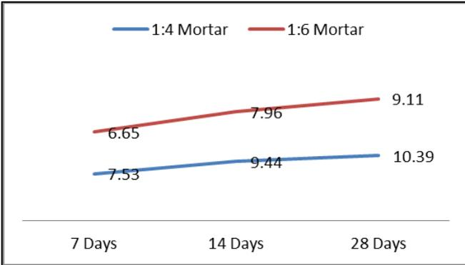
Fig. 8: Comparison of compressive strength of 1:4 and 1:6 cubes with bottles arranged Parallel to the direction of load application
