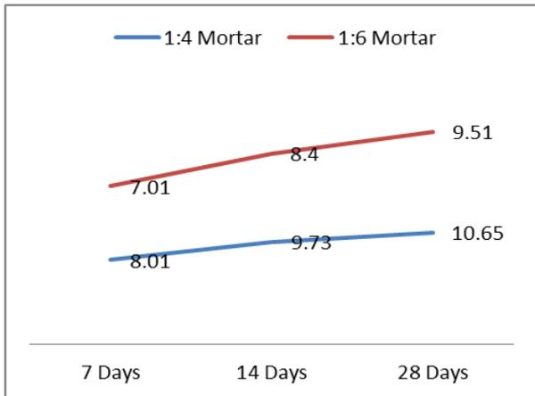
Fig. 6: Comparison of compressive strength of 1:4 and 1:6 cubes with bottles arranged Parallel to the direction of load application
