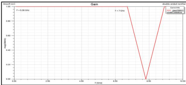
Fig. 5: Gain Plot of Double-Sided Rectifier
