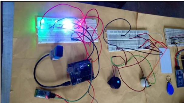
Fig. 3: Bluetooth HC-05 Operating at Breadboard
