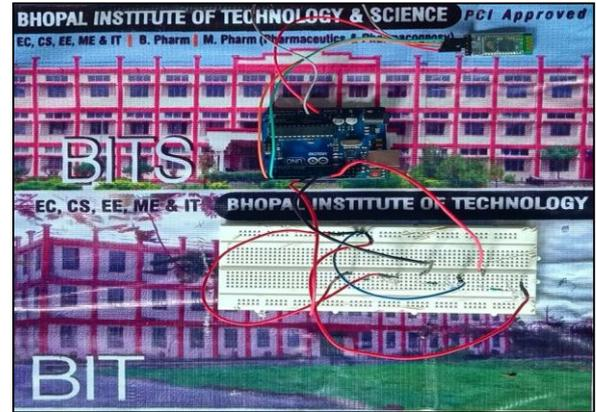
Fig. 4: Bluetooth HC-05 Breadboard Setup
