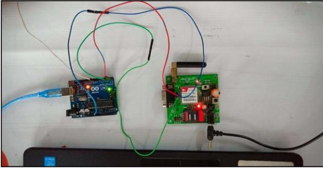
Fig. 5: GSM-Arduino UNO based Automation
