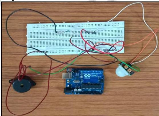
Fig. 9: PIR-Arduino based Automation Setup
