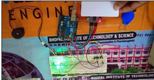
Fig. 2: RFID accepted Card
