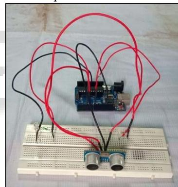
Fig. 10: Ultrasonic Sonic Sensor with Arduino
