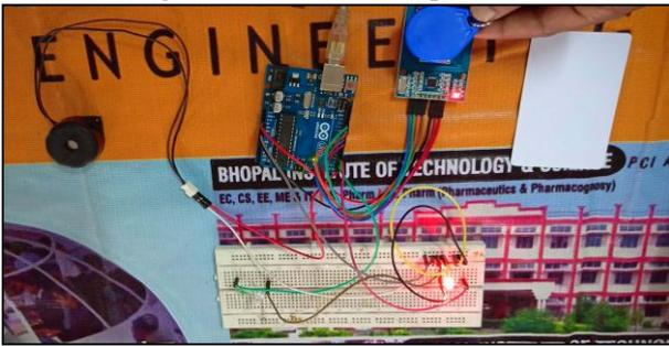
Fig. 1: RFID not accepted Card
