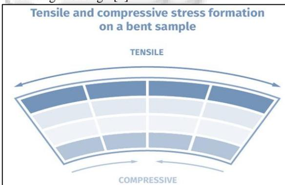
Fig. 1: Tensile & Compressive Stress Formation on Bent Sample
