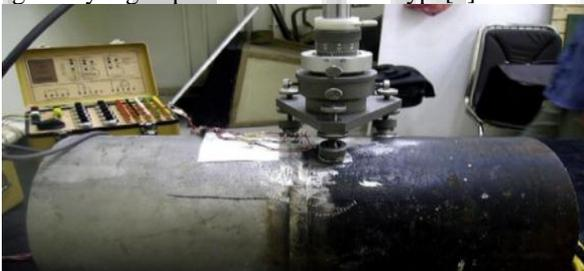
Fig. 3: Experimental Setup of Hole Drilling Method
