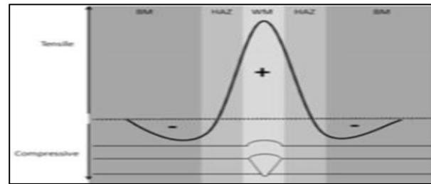
Fig. 5: Welding Residual Stress Distribution
