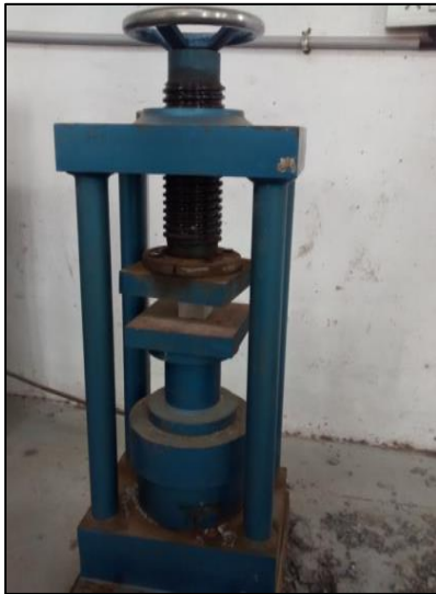
Fig. 2: Compression testing of cement cube
