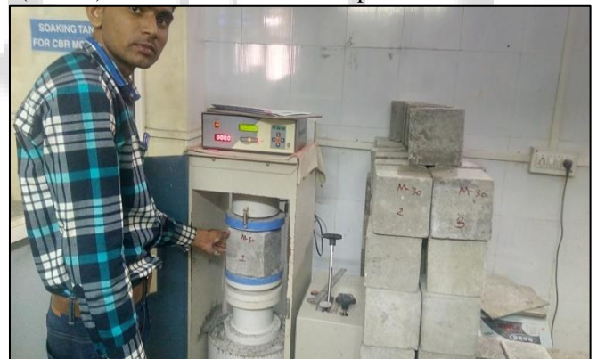
Fig. 3: Compressive strength test of concrete
