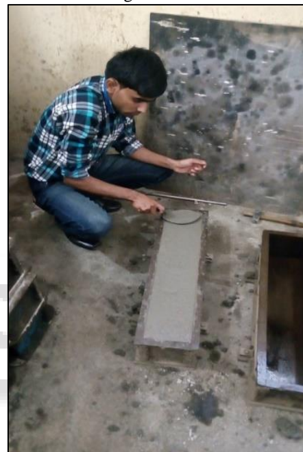
Fig. 7: Casting of reinforced beam
