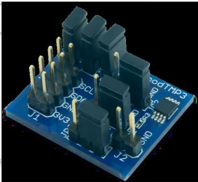
Fig. 1: Pmod TMP3 - Temperature Sensor
