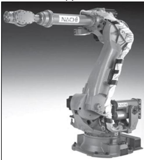
Fig. 1: An Industrial Robotic Manipulator for Stacking Bags on a Pallet. Image Courtesy of Nachi Robotic Systems
