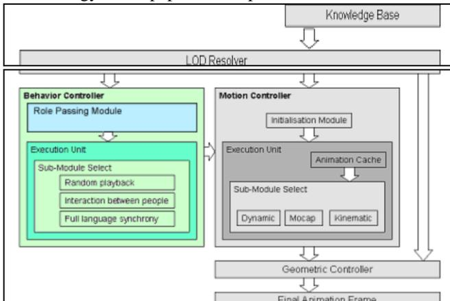
Fig. 1: Original ALOHA Framework Extended to Incorporate Role-Passing into the Behavior Controller [5]
