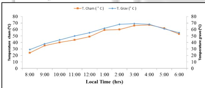
Fig. 1.4: Drying Chamber & Grave Temperature
