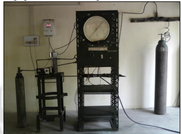
Fig. 1: High Pressure Strand Burner setup
