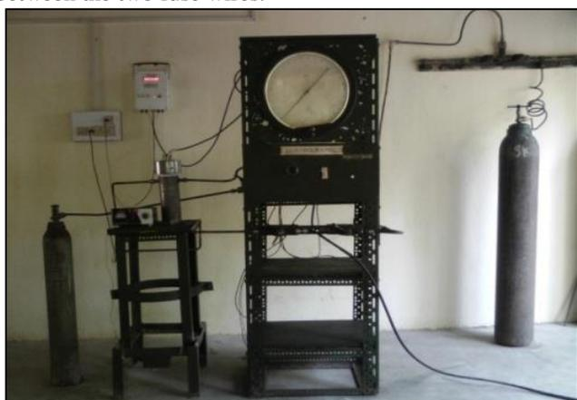
Fig. 1: High Pressure Strand Burner Setup
