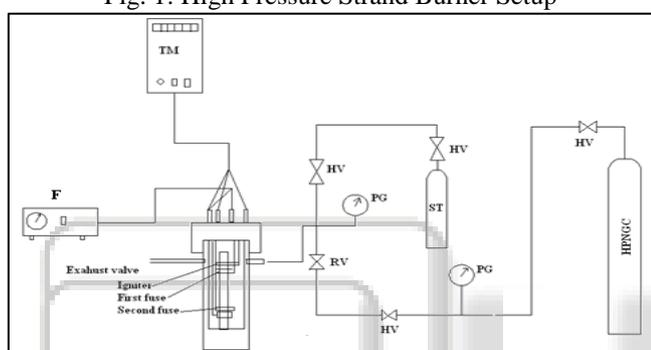
Fig. 2: Line Diagram of High Pressure Strand Burner
