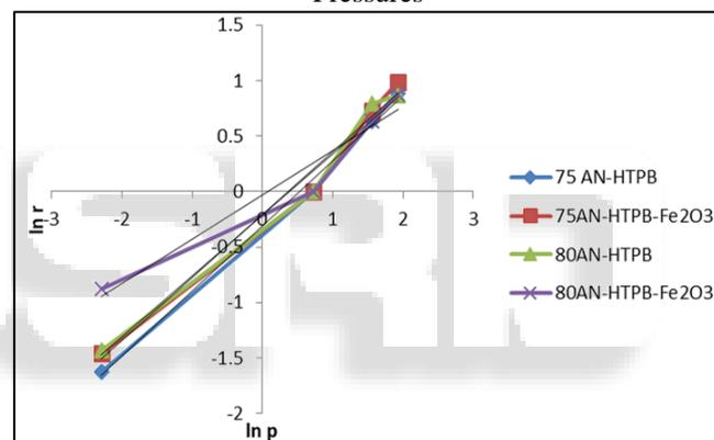
Fig. 3: Comparison of Burning Rate 70, 75 & 80% of AN-HTPB Composite Solid Propellant with Catalyst
