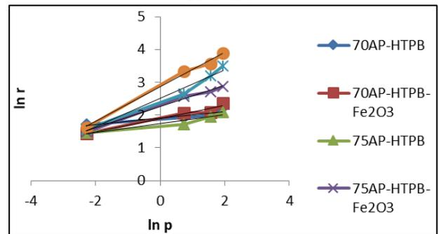
Fig. 3: Comparison of Burning Rate 70, 75 & 80% of AP-HTPB Composite Solid Propellant with Catalyst
