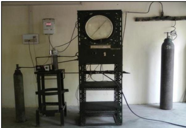
Fig. 1: High Pressure Strand Burner Setup
