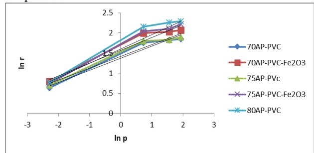
Fig. 3: Comparison of Burning Rate 70, 75 & 80% of AP-PVC Composite Solid Propellant with Catalyst
