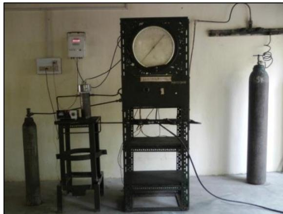
Fig. 1: High Pressure Strand Burner Setup
