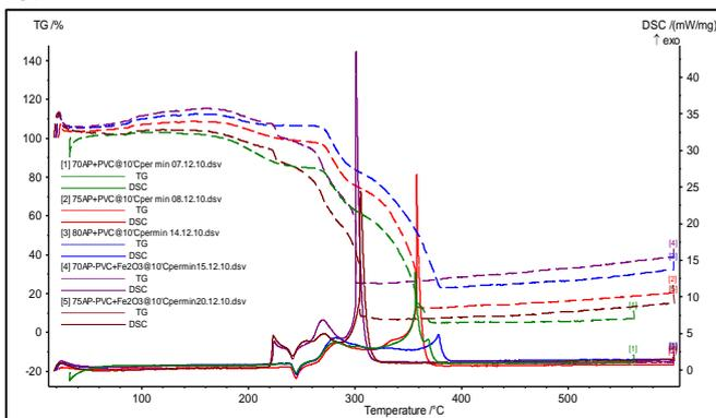
Fig. 3: Comparison of STA graph showing DSC/TG of AP - PVC composite solid propellant
