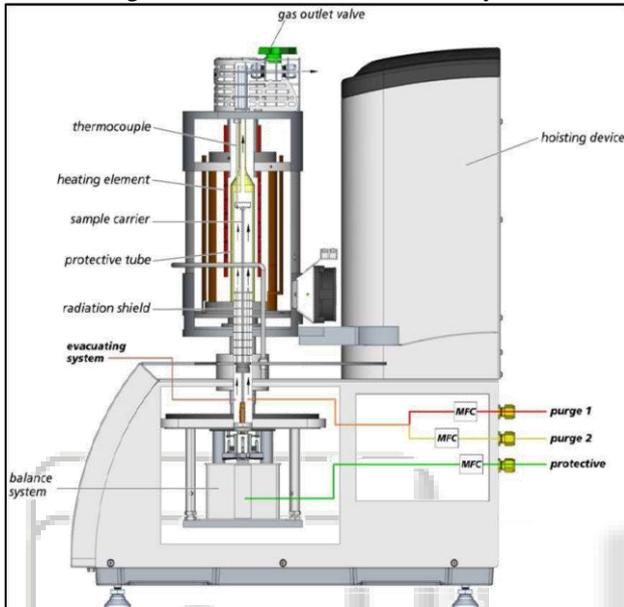
Fig. 2: Internal Structure of the Simultaneous Thermal Analyzer
