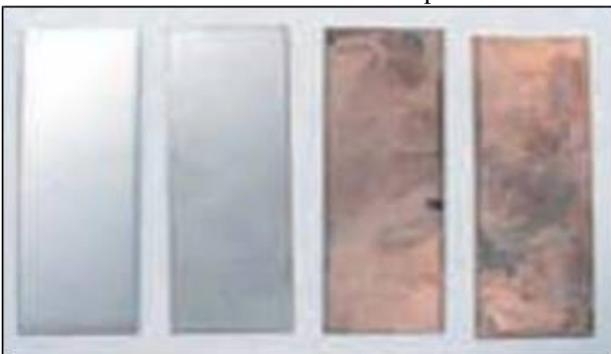
Fig. 5.1: PEEK & SS316L after Corrosion Test
