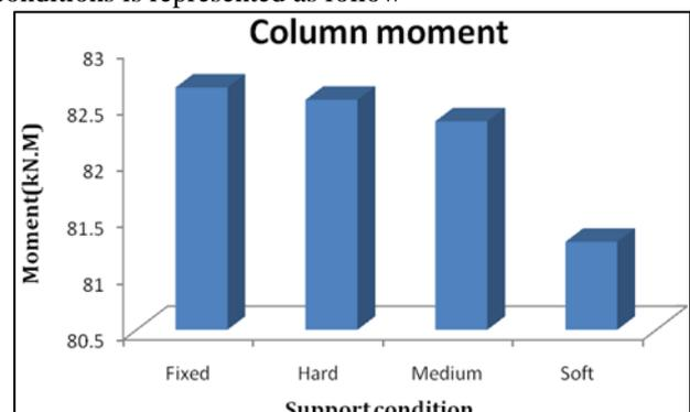
Fig. 12: Column Moment for Different Soil
