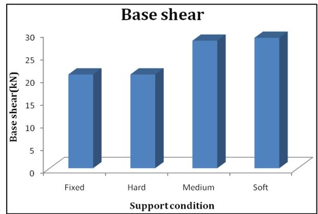
Fig. 10: Base Shear for Different Soils
