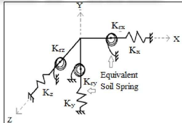
Fig. 9: Equivalent Spring Stiffness
