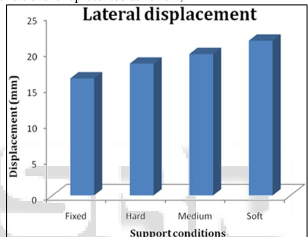
Fig. 11. Lateral displacement for various soils
