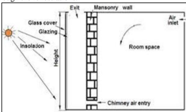
Fig 1: Schematic of Solar Chimney
