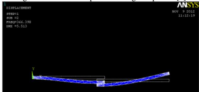
Fig. 5: Second Mode Shape Al-Al Single Lap Joint [6]
