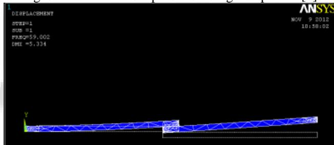
Fig. 4: First Mode Shape Al-Al Single Lap Joint [6]
