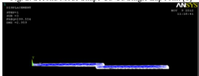
Fig. 3: Third Mode Shape Cu-Cu Single Lap Joint [6]
