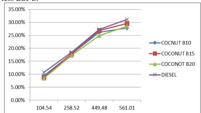
Fig. 6: BMEP (Kpa) vs BTE
