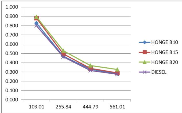
Fig. 7: BMEP (Kpa) vs BSFC (Kg/KW-hr)
