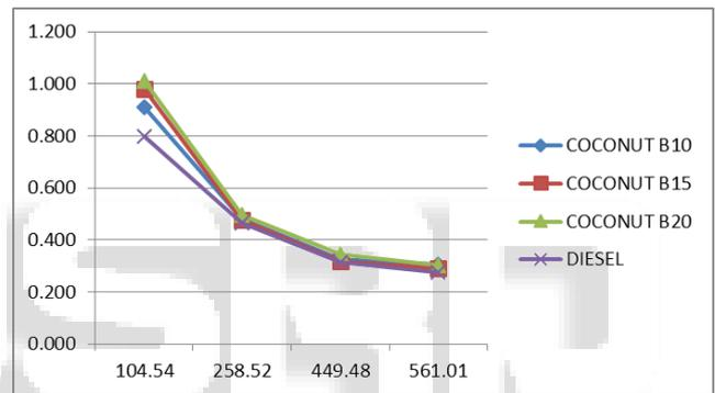
Fig. 5: BMEP (Kpa) vs BSFC (Kg/KW-hr)
