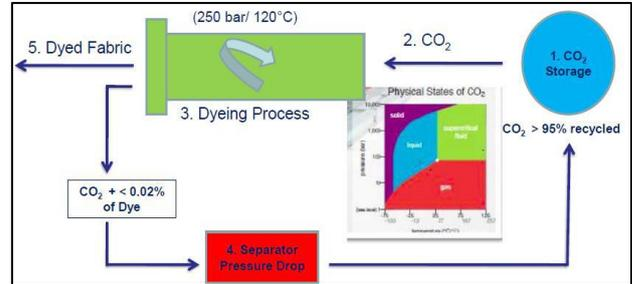
Fig. 5: SFC Dyeing Apparatus
