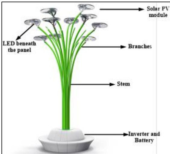
Fig. 2: Layout of Solar Tree
