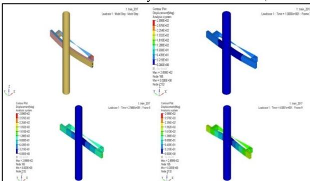
Fig. 4: Crash Test Performed on Simple bumper Beam
