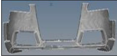
Fig. 3: Mesh Model of Bumper
