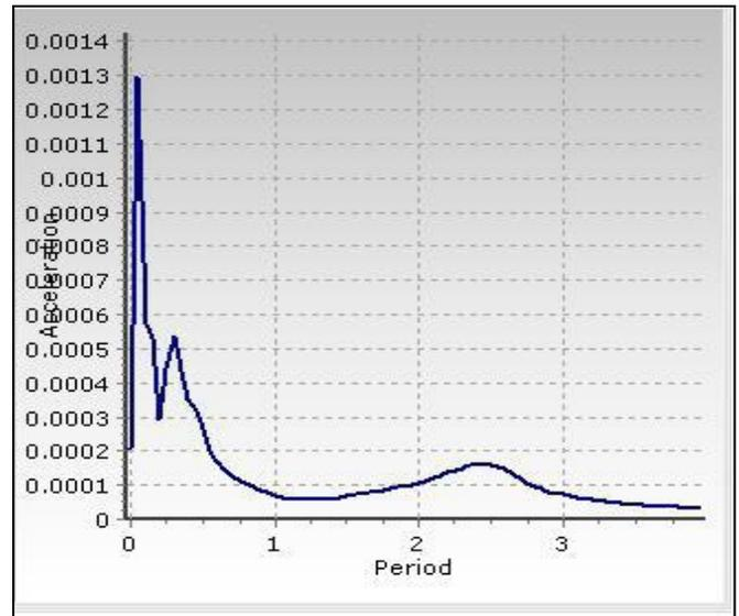
Fig. 4: Response spectrum curve (Fault normal)
