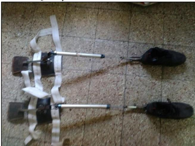
Fig. 1: Experimental setup of Chair less seating
