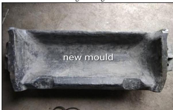
Fig. 1: Pig casting machine mould
