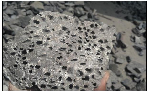
Fig. 6: Surface Blows on the Casting
