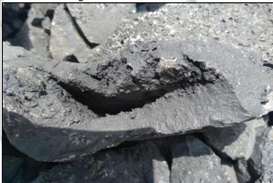
Fig. 7: Unsolidified Cavity in PCM Casting
