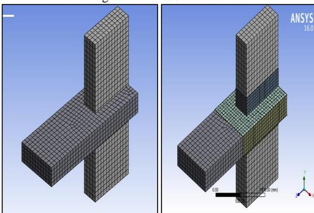
Fig. 3: meshing of exterior wide beam column joint without FRP and with FRP using ANSYS
