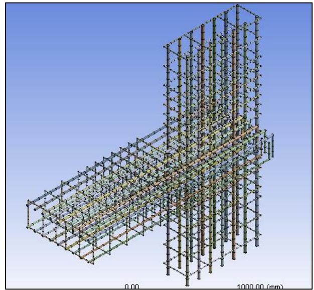
Fig. 4: Detailing of specimen as per IS 13920:1993
