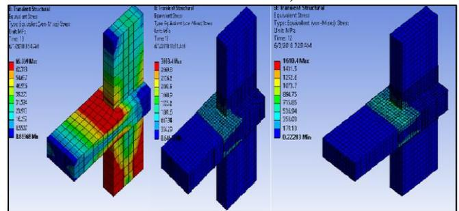
Fig. 10: equivalent stress without FRP, with CFRP and GFRP
