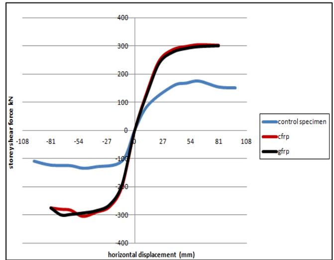
Fig. 9: shear force – displacement graph (without FRP, with CFRP and GFRP)
