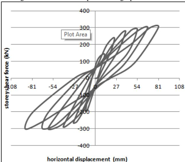
Fig. 8: shear force displacement graph with GFRP
