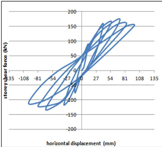
Fig. 6: shear force – displacement graph without FRP
