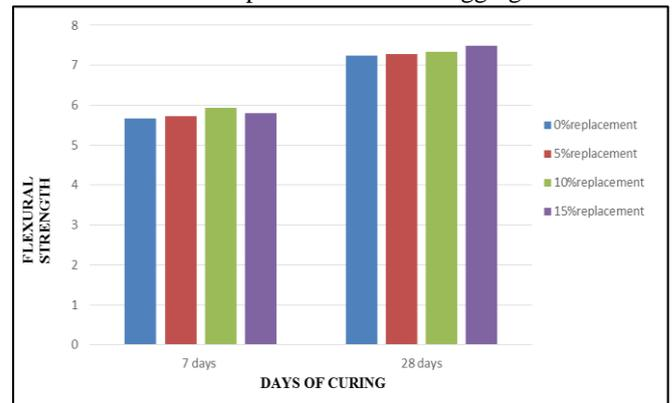
Fig 4.3: Variation of Flexural Strength at 7 and 28 days for M20 grade concrete & concrete mix with 5%, 10% and 15% crumb rubber as replacement for fine aggregate
