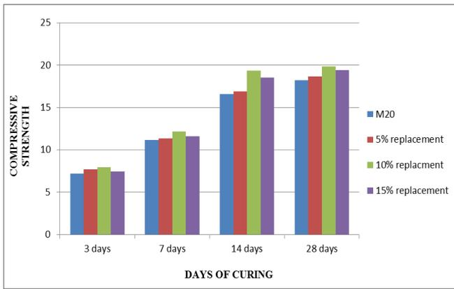
Fig 4.2: Variation of Compressive Strength at 3, 7, 14 and 28 days for M20 grade concrete & concrete mix with 5%, 10% and 15% crumb rubber as replacement for fine aggregate
