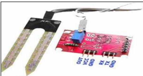
Fig. 2: Soil Moisture Sensor
