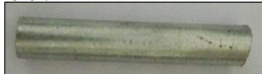
Fig. 2: Aluminium 6061 Billets used as a Base Material
