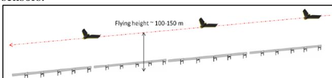
Fig. 4: Long Distance Survey with Automatic Sensing of Soil Properties [10]
