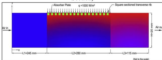
Fig. 3.3.1: Sketch of the Computational Domain of Rectangular Rib Section
