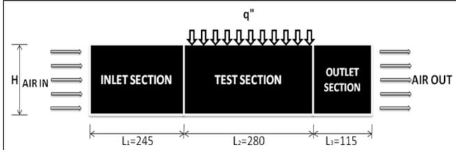
Fig. 3.1: Schematic Diagram of the Investigated Region of Smooth Rectangular Channel
