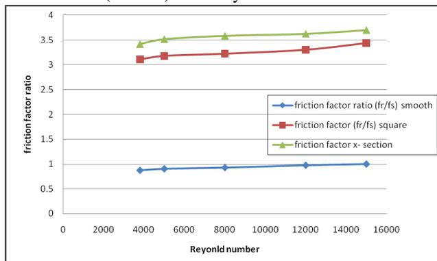
Fig. 5.3.2: Variation of friction factor ratio,  $f_{rib}/f_{smooth}$  with Reynolds number
