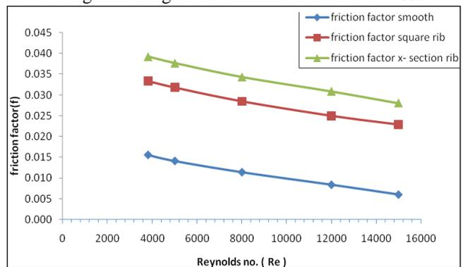
Fig. 5.2.2: Variation of Friction factor (f) with Reynolds Number for Various Rib Shapes
