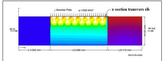
Fig. 3.4.1: Sketch of the Computational Domain of Rectangular Rib Section
