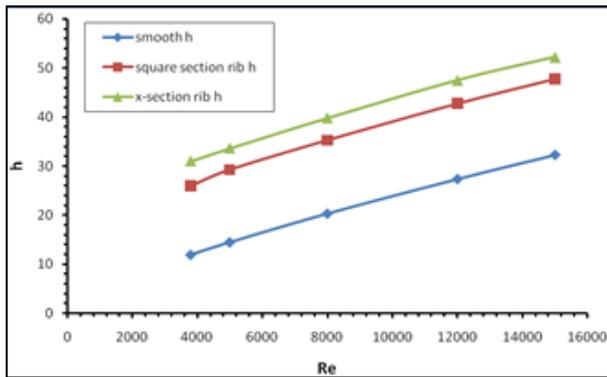
Fig. 5.3.5: Variation of Convection Heat Transfer Coefficient (h) with Reynolds No
