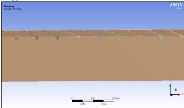
Fig. 3.3: Schematic Diagram of Rib Geometry (Rectangular Section)
