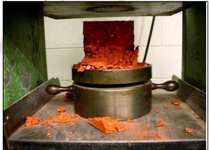
Fig. 4: compression testing of brick
