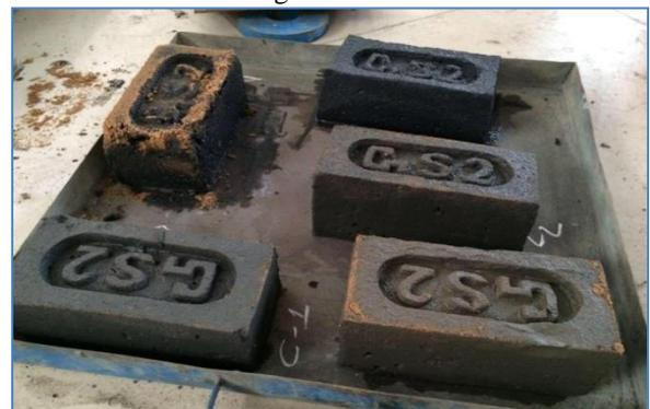
Fig. 2: Brick sample shape and size after moulding
