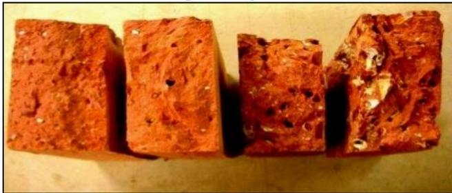
Fig. 6: cross section of brick having different percentage of cigarette butt content i.e.5%,10%, 15% and 20%
