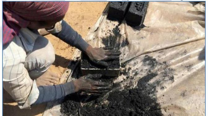
Fig. 1: manufacturing of brick with varying percentage of cigarette butt
