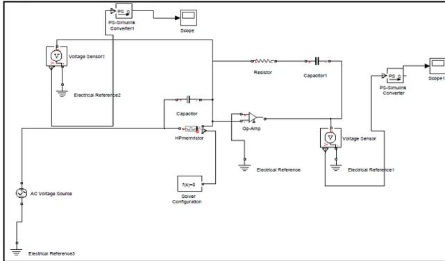
Fig 11: Simulation Model of Memristor Element Based PID Controller
