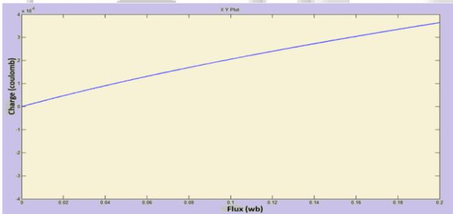
Fig. 7: charge Vs flux characteristic of Memristor
