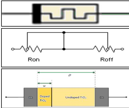
Fig. 2: Circuit Symbol & Device Structure of Memristor
