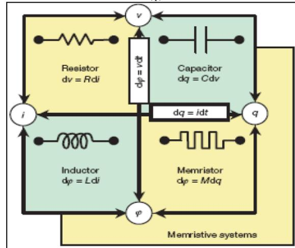
Fig. 1: Fundamental Circuit Element Relations
