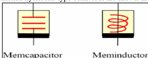
Fig 13: Memcapacitor & Meminductor
