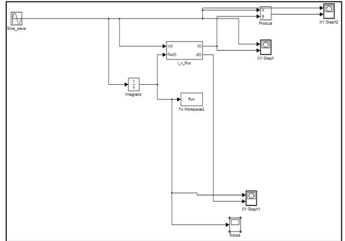
Fig 3: Simulink Model of Memristor
