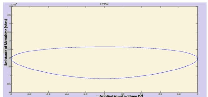
Fig. 5: Resistance Vs Input Voltage of Memristor
