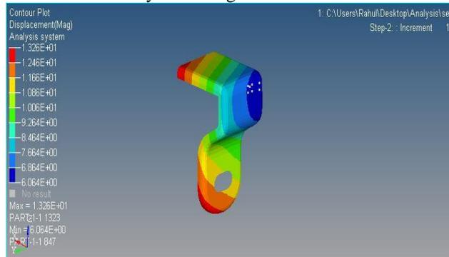
Fig. 7: Displacement of Existing Bracket
