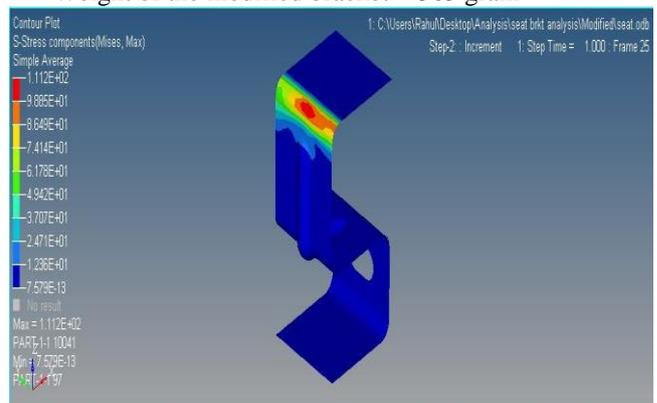
Fig. 10: Stress of Modified Bracket
