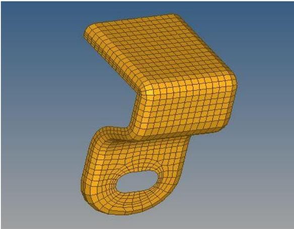
Fig. 5: Meshing of Existing Bracket
