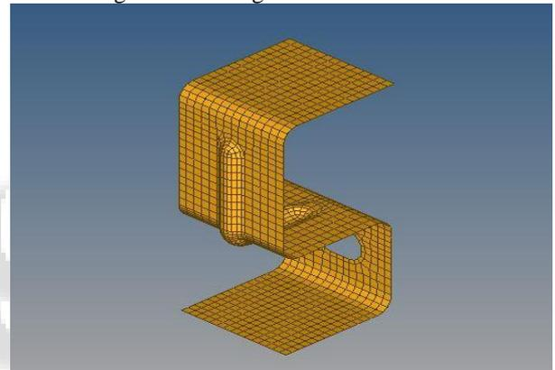
Fig. 9: Meshing of Modified Bracket
