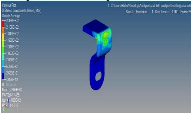
Fig. 6: Stress of Existing Bracket
