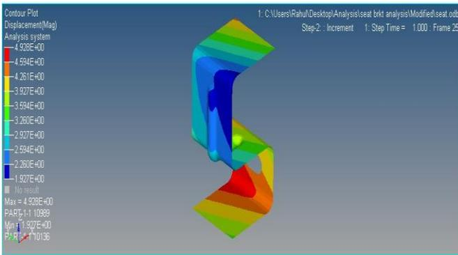
Fig. 11: Displacement of Modified Bracket
