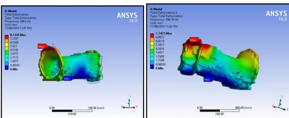
Fig. 10: Mode shapes of structural steel
