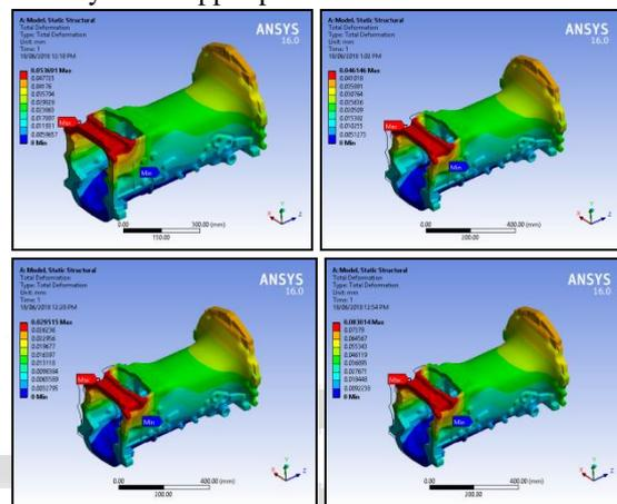
Fig. 7: Total deformation of different material
