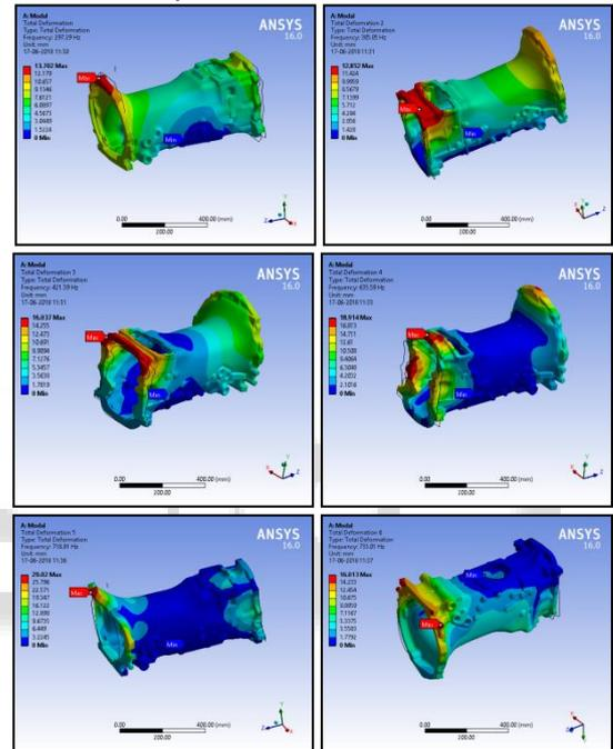
Fig. 11: Mode shapes of aluminum alloy
