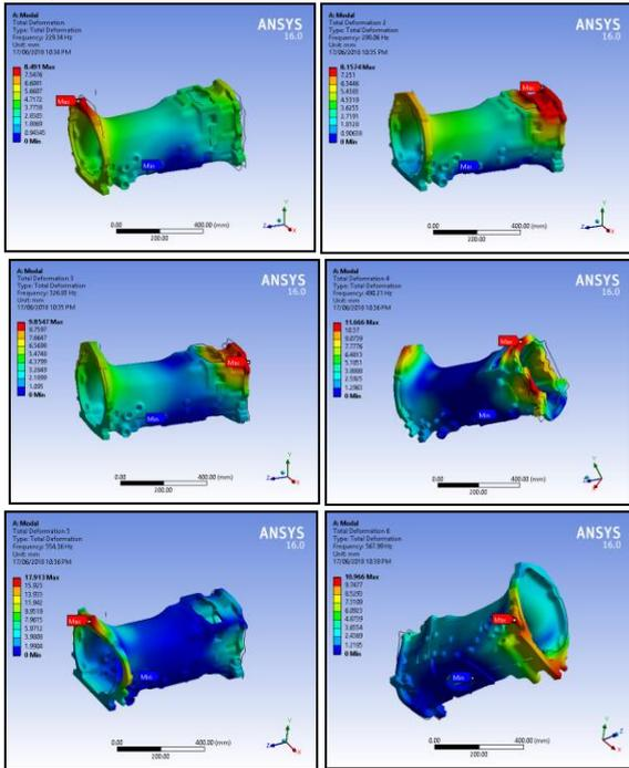
Fig. 8: Mode shapes for FG220
