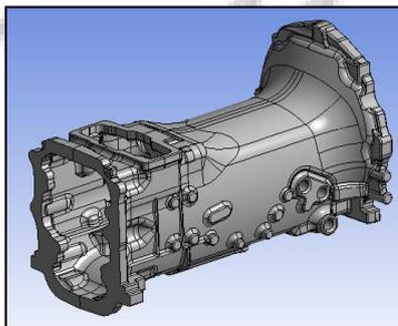
Fig. 1: Transmission housing
