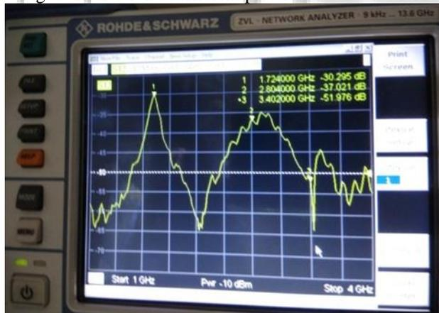
Fig. 7: Transmission coefficient practical result on VNA
