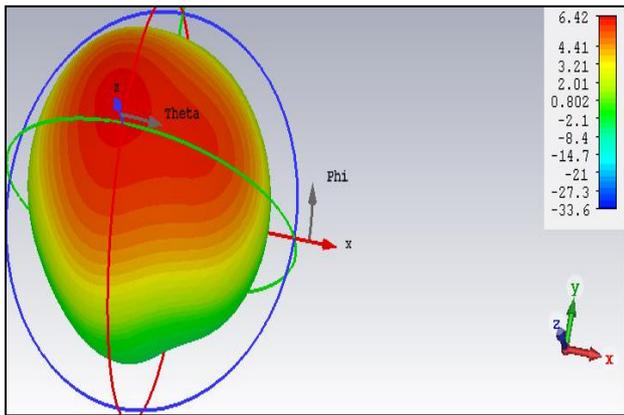
Fig. 11: radiation pattern at 2.7GHz
