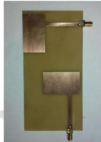
Fig. 3: Fabricated 2 element MIMO antenna
