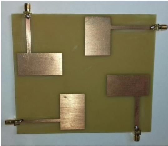
Fig. 5: Fabricated 4 element MIMO antenna.
