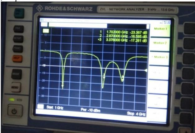
Fig. 6: Reflection coefficient practical result on VNA
