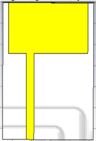
Fig. 1: Simple microstrip patch antenna design
