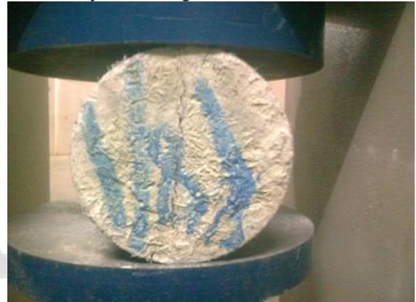
Fig. 2: Split Tensile Strength Test
