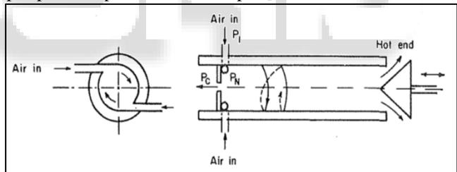
Fig. 3: Schematics of The Ranque-Hilsch vortex Tube.
