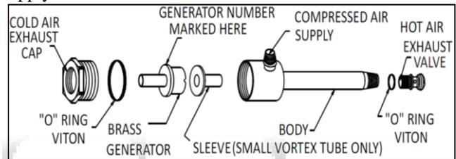
Fig. 2: Parts detail of Vortex Tube [NEXFLOW]
