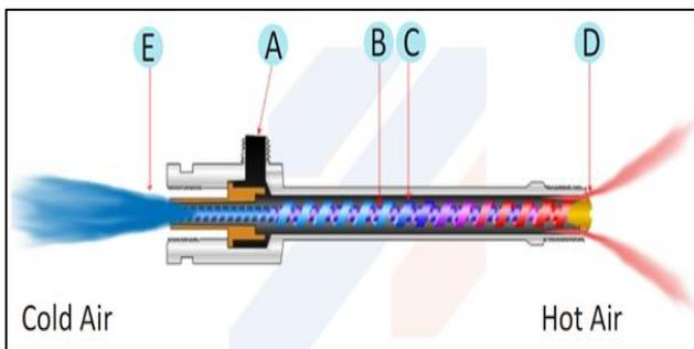
Fig. 1: Working of Vortex Tube [NEXFLOW]
