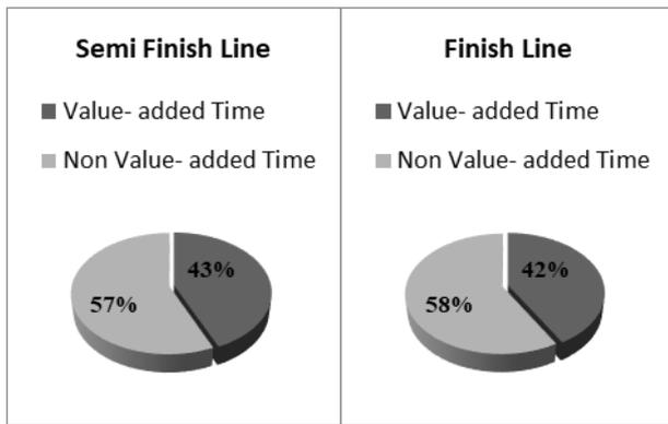
Fig. 4: Pie Chart for VA & NVA Time for Semi Finish & Finish Lines
