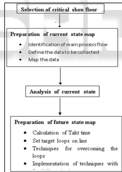
Fig. 1: Steps of Value Stream Mapping
