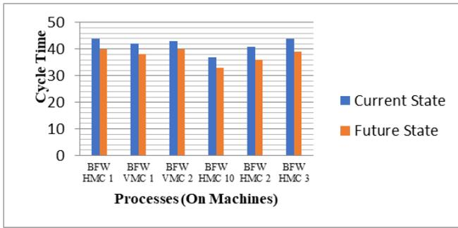
Calculation of Total Lead Time directly depends on two parameters the cycle time and the inventory for each work station. With reduced cycle time and ideal condition of inventory for each process the reduction observed in lead time is summarized in table: 2.
