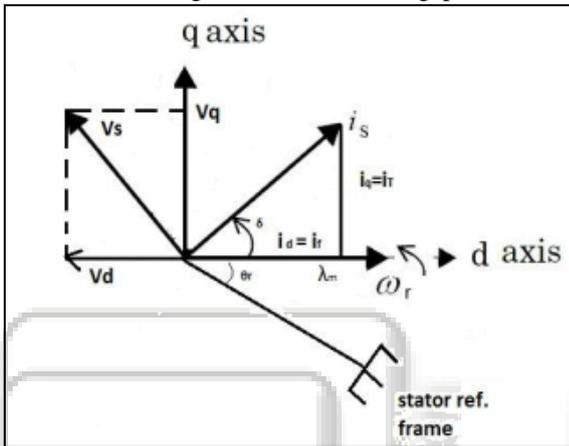
Fig. 2: Phasor diagram of PMSM
