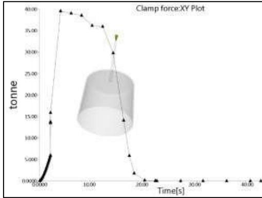
Fig. 12: Clamp Force Require for the Cycle
