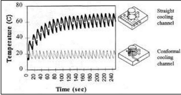
Fig. 3: Comparison of Mold Surface Temperature Histories for Straight Channel Cooling & Conformal Channel Cooling
