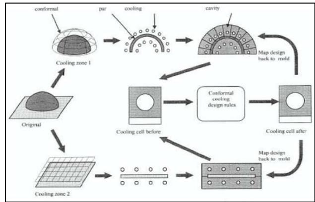
Fig. 2: Steps for the Modularized Cooling Line Design for a Generic Part
