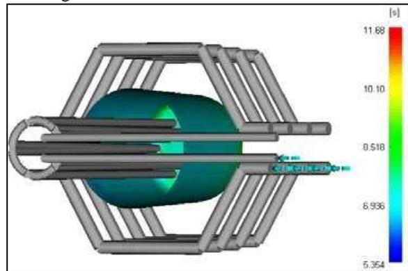
Fig. 15: Part's Cooling Time
