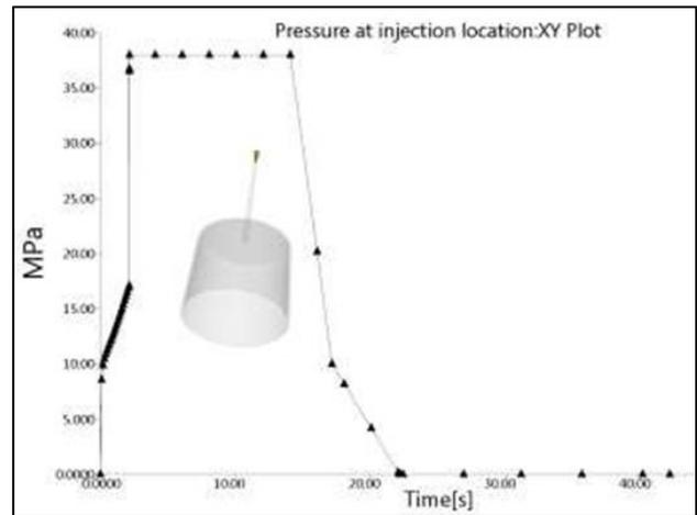
Fig. 9: Pressure at Injection Location
