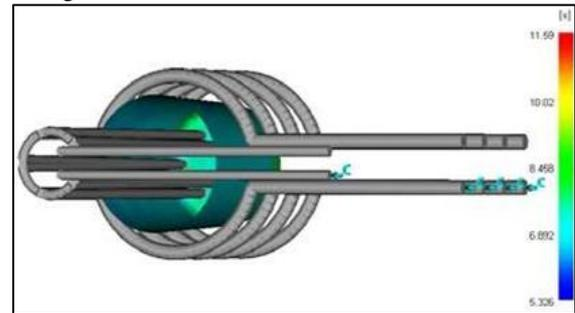
Fig. 23: Part's Cooling Time
