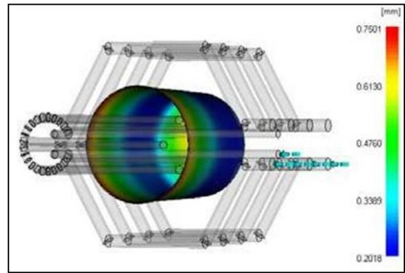
Fig. 14 Part's Deflection the Part's Surfaces
