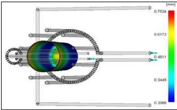
Fig. 18: Part's Deflection on the Part's Surfaces
