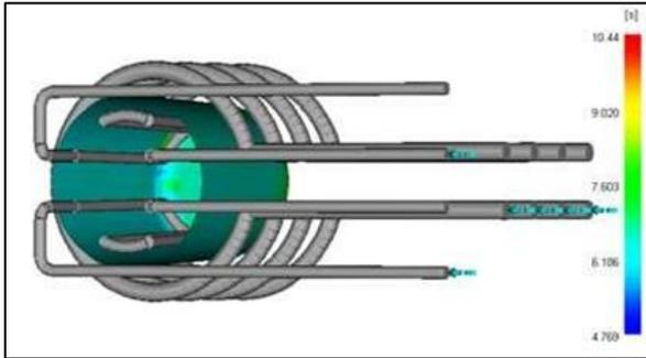
Fig. 27: Part's Cooling Time
