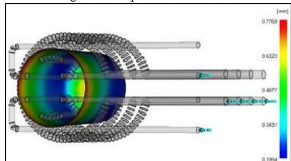
Fig. 26: Part's Deflection on the Part's Surfaces
