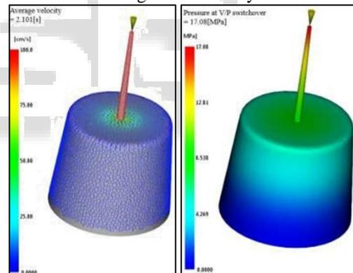
Fig. 10: Average Velocity Fig. 11: Pressure Switch Over
