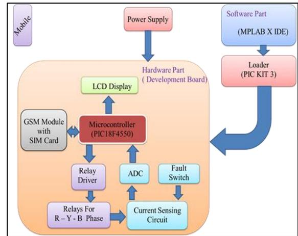
Fig. 2.1: Block Diagram of Complete Project
