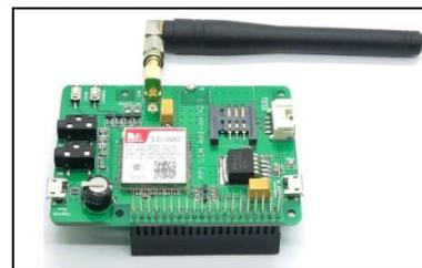
Fig. 2.2: SIM 800 GSM Modem
