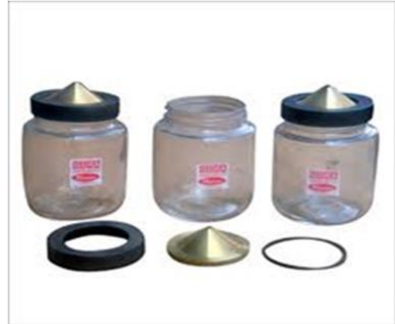
Fig. 1: Specific gravity test for fine Aggregate
