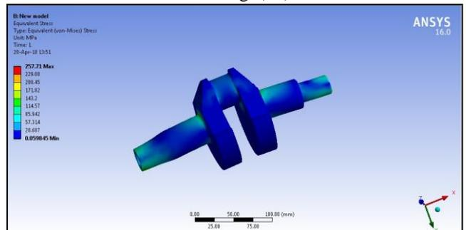
Fig. 13: Max Strain in Crankshaft
