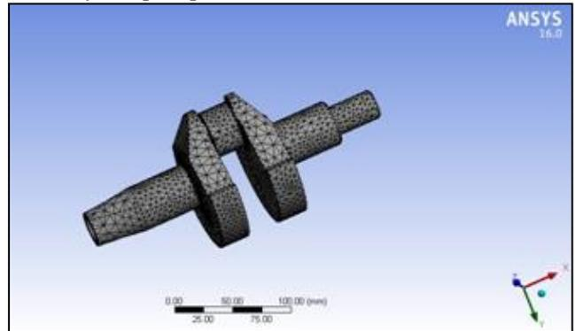
Fig. 5: Meshing of Crankshaft Model
