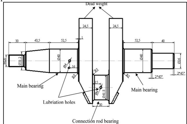
Fig. 2: Crankshaft Design
