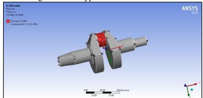
Fig. 7: Force Apply on Crankshaft Model
