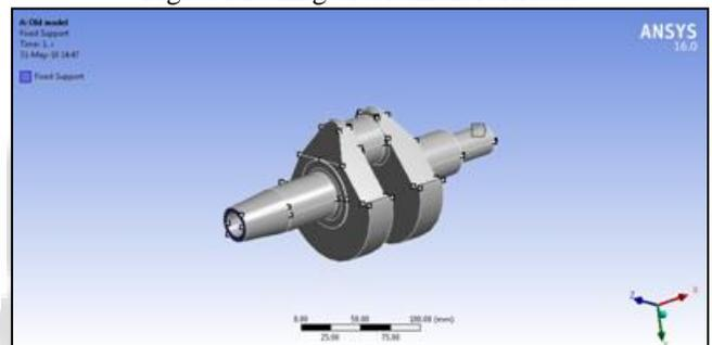
Fig. 6: Fixed Support of Crankshaft Model
