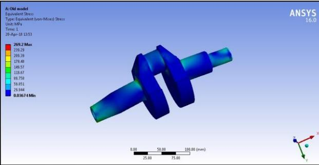
Fig. 9: Max Stress in Crankshaft
