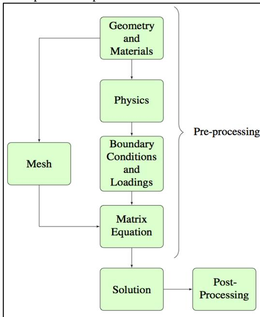
Fig. 4: Finite Element Analysis procedure
