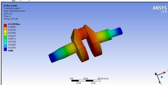
Fig. 11: Max Deformation in Crankshaft
