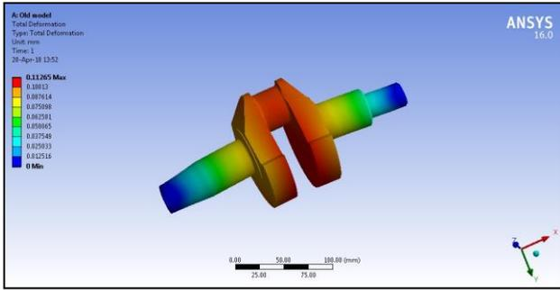
Fig. 8: Max Deformation in Crankshaft
