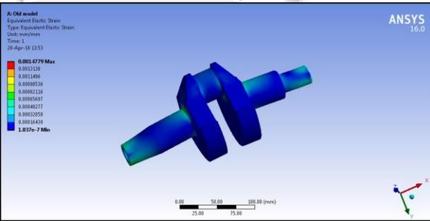
Fig. 10: Max Strain in Crankshaft
