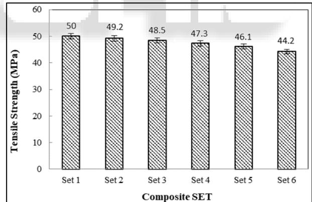
Fig. 2: Tensile Strength of Epoxy/SGM Composites
