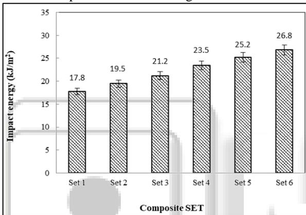
Fig. 4: Impact Energy of Epoxy/SGM Composites
