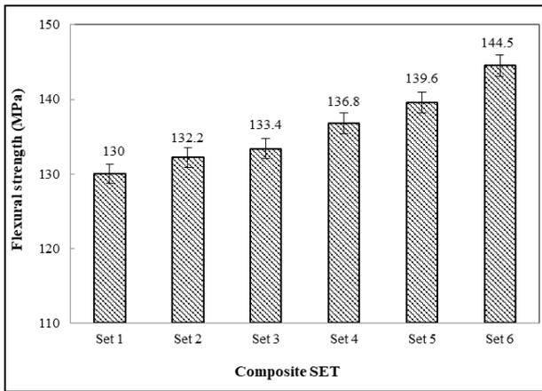
Fig. 3: Flexural Strength of Epoxy/SGM Composites
