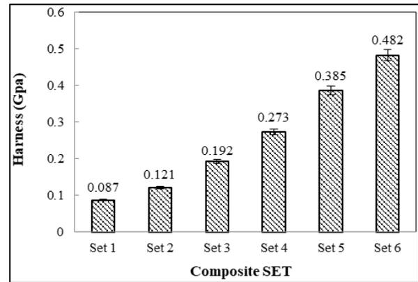
Fig. 1: Micro-Hardness of Epoxy/SGM Composites
