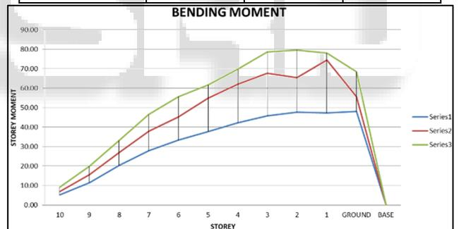
Table & Graph 6.43: Max Bending moment Comparison for Response spectrum For Soil-I
