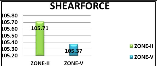
Table & Graph 6.19: Max Shear force Comparison for 1.2(DL+LL+EQY) for Soil-II
