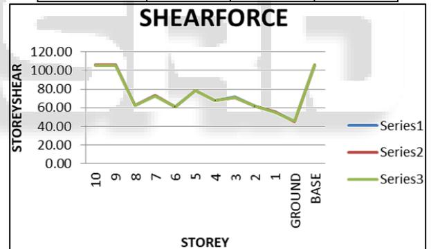
Table & Graph 6.13: Showing Storey Shearforce for 1.2(DL+LL+EQX) for Zone-V
