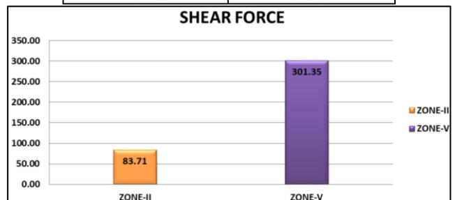
Table & Graph 6.39: Max Shear force Comparison for Response spectrum for Soil-II
