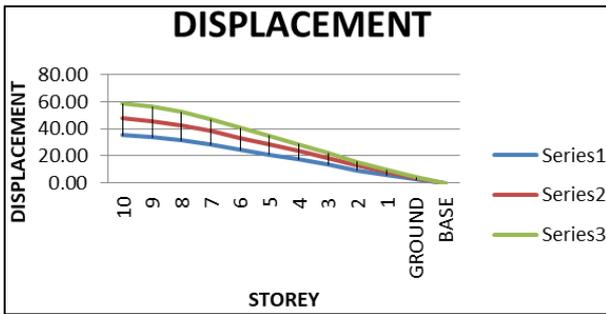
Table & Graph 6.4: Showing Storey Displacement for 1.2(DL+LL+EQY) for Zone-V
