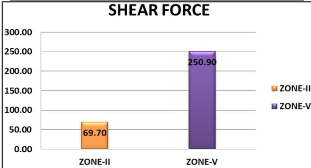
Table & Graph 6.40: Max Shear force Comparison for Response spectrum for Soil-III
