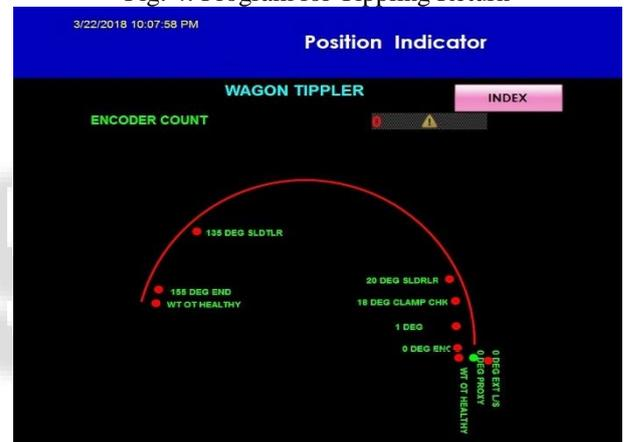
Fig. 5: Operator Interface at HMI
