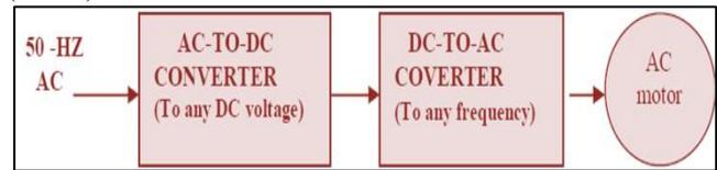
Fig. 1: Block Diagram of Speed Control Method
