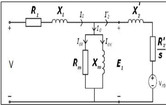
Fig. 2: Equivalent to Circuit of Poly Phase Induction Motor
